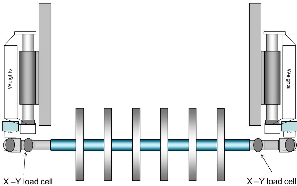
**Figure 9.** The framework to which the gear components and axle were attached showing where the additional weights were fitted and the position of the two Strainstall 500kg X-Y load cells.
