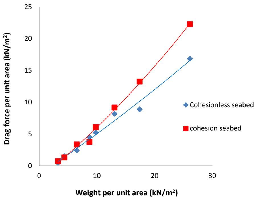
**Figure 13** Comparison between cohesive and non-cohesive soil
