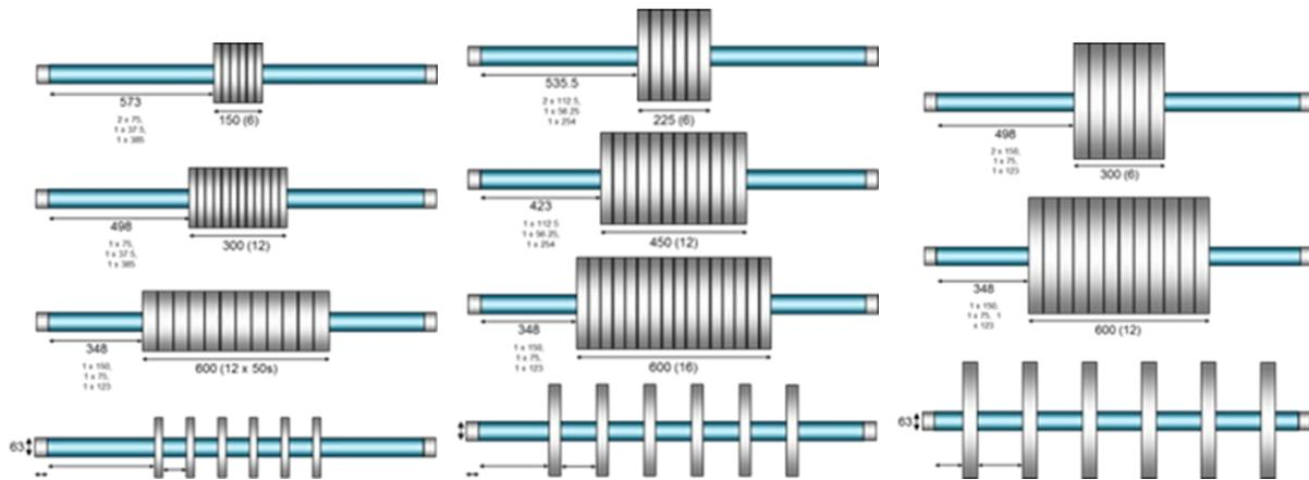
**Figure 8.** The range of gear components chosen to simulate some of the groundgears and clump weights used in demersal fisheries comprising disks and cylinders of diameter 200, 300 and 400mm.
