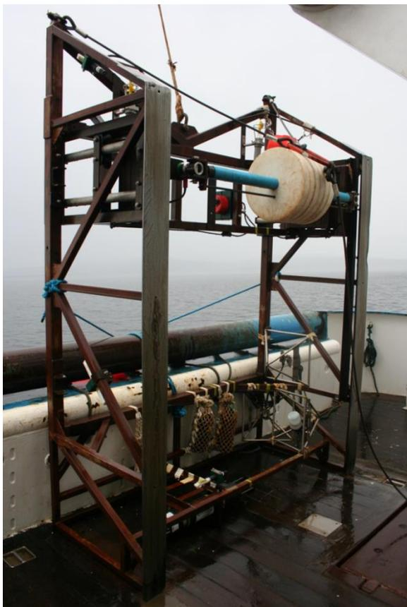
**Figure 7.** The towed sledge used to tow the range of cylindrical objects supported on an axle.
