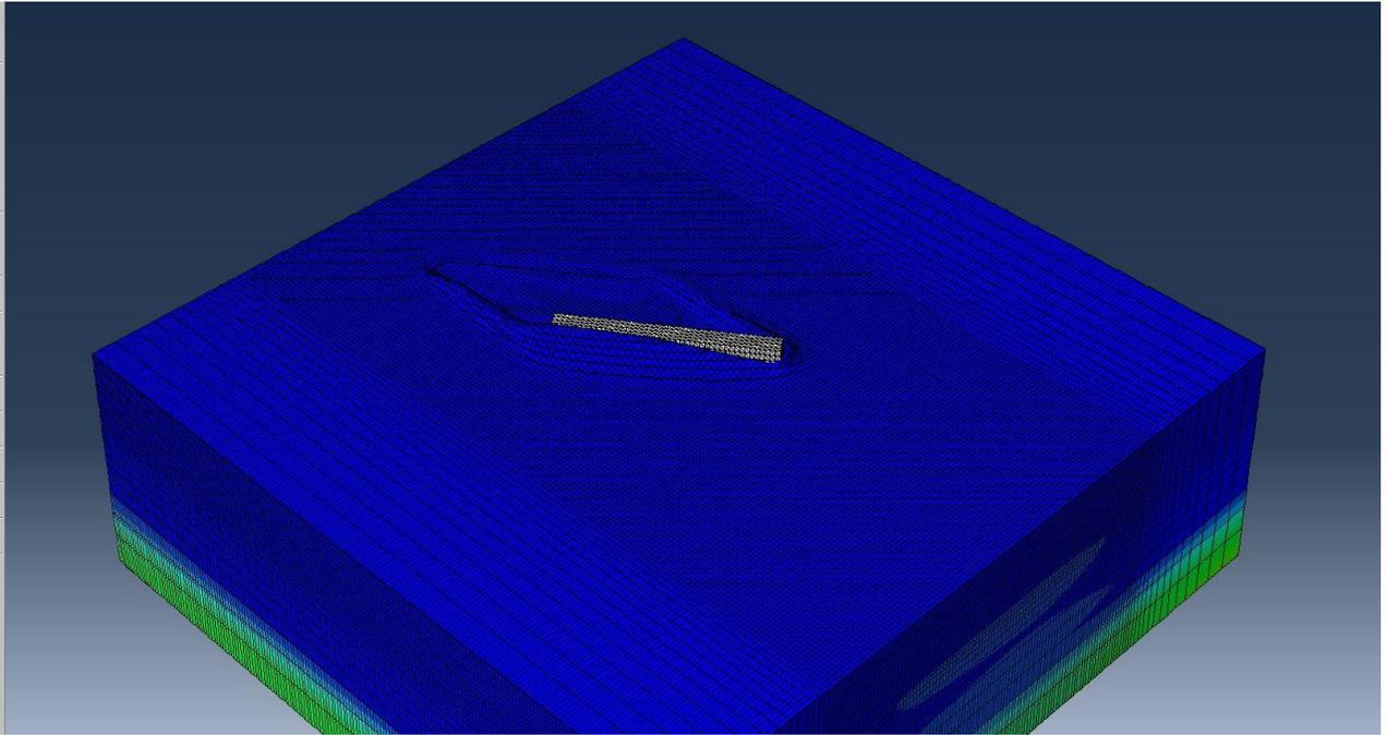
**Figure 5** An image from Abaqus ( otter door shoe on sandy sediment)
