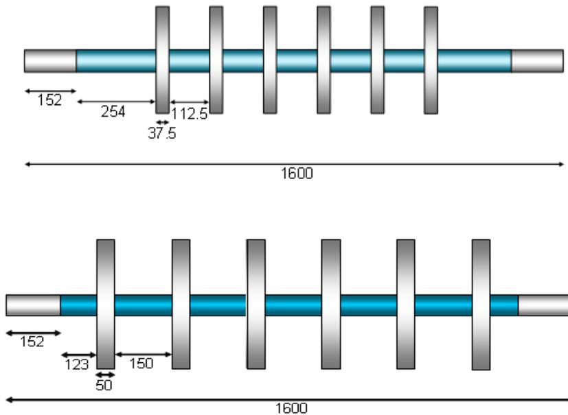
**Figure 3** Schematic view of the ground gear assemblies (200mm dia of the top and 400mm dia of the bottom)
