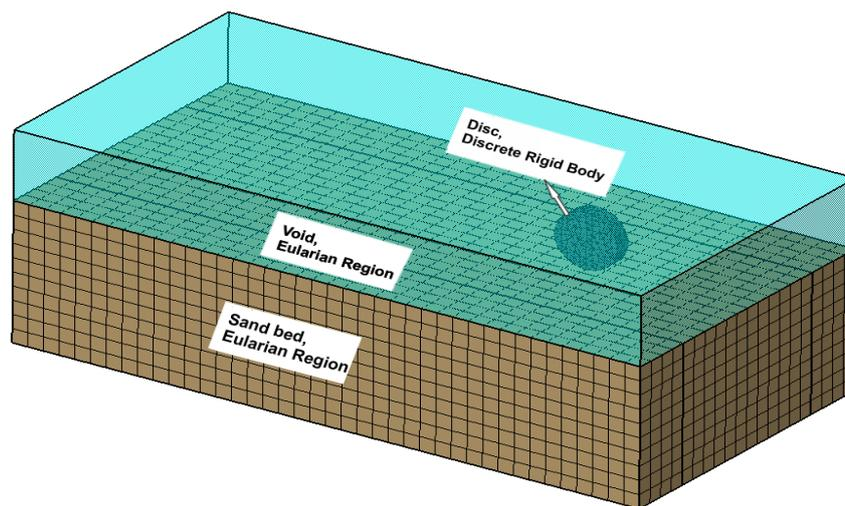
**Figure 1** schematic representation of the FE model
