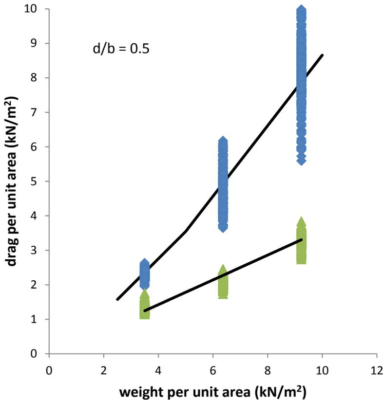
**Figure 14** Comparison between cohesive and non-cohesive soils
