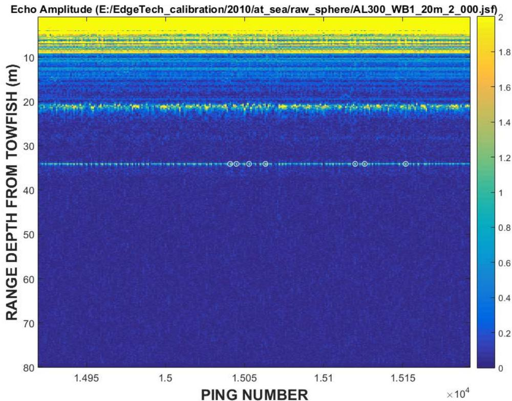
Figure 11. First output diagram obtained running the `plot2d_color` script during calibration. Selected pings are circled in white. It is important to know the position of the calibration sphere as noise inherently present in the system can produce confusing results (the banding seen from the 20m mark upward is such an artefact).
