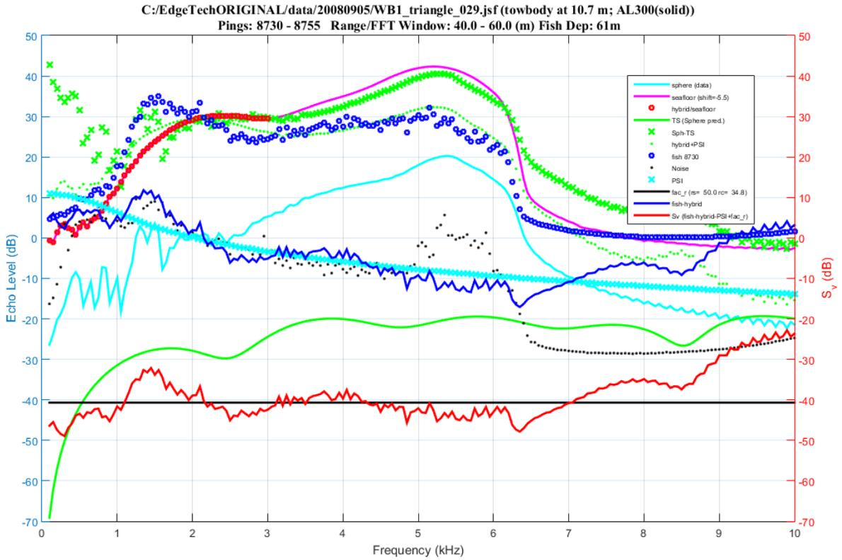
Figure 14. First output of Sv\_diag\_2010. This plot shows details of the various component elements that go into the final VBS result. The VBS result itself is the solid red line.
