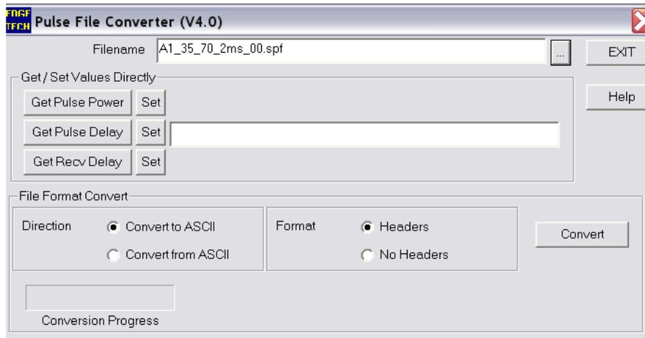
Figure 6. Pulser program used to convert EdgeTech 3200 pulse files into ones compatible with the Matlab based processing software.
