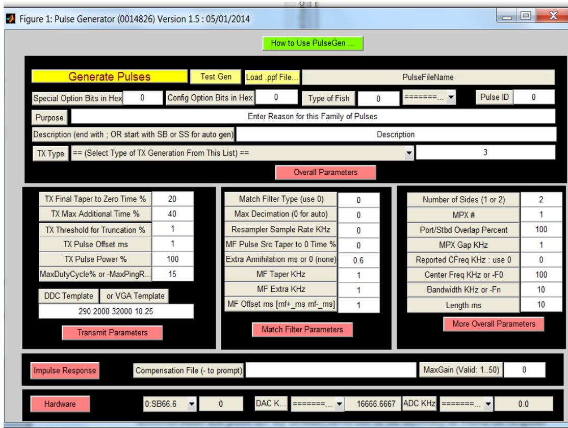
Figure 5. GUI interface of program used to generate signal files for MSS EdgeTech 3200
