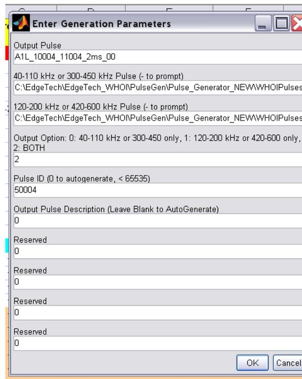
Figure 7 WSEPulse program, used for combining two AirMar pulse files into one in a process called 'mangling'.
