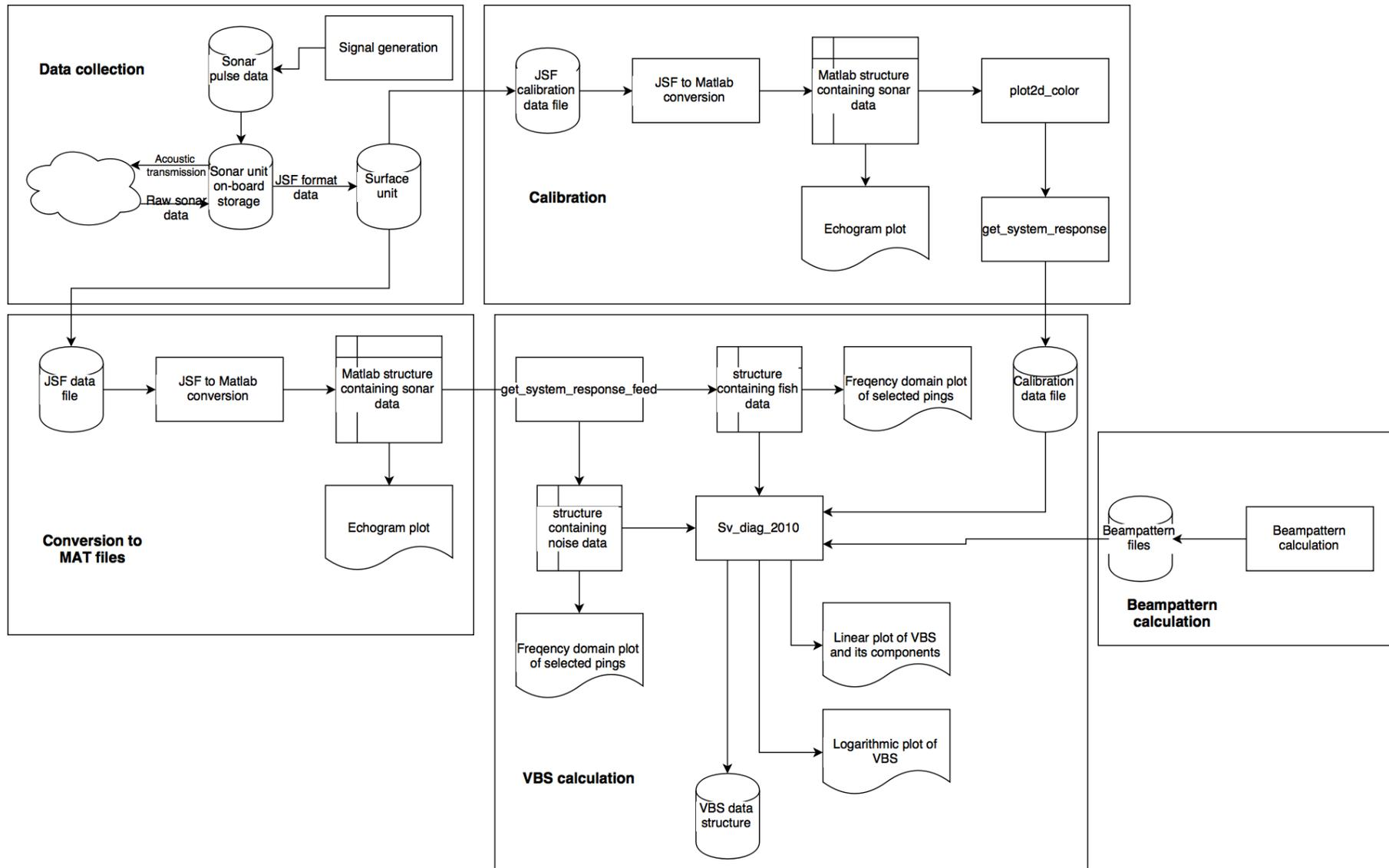
Figure 4. Data flow diagram for the EdgeTech 3200 system covering data collection and processing.
