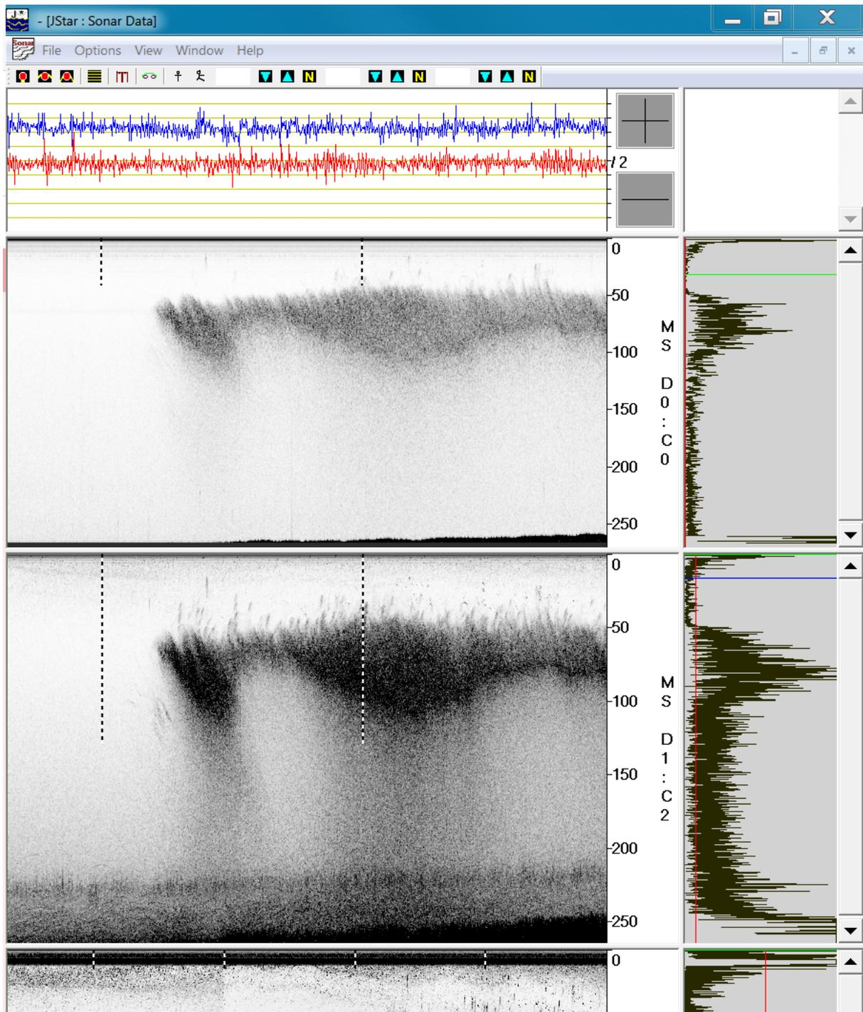
Figure 9. Main graphical display of JSTAR program used to collect and playback acoustic data from the EdgeTech 3200 system.
