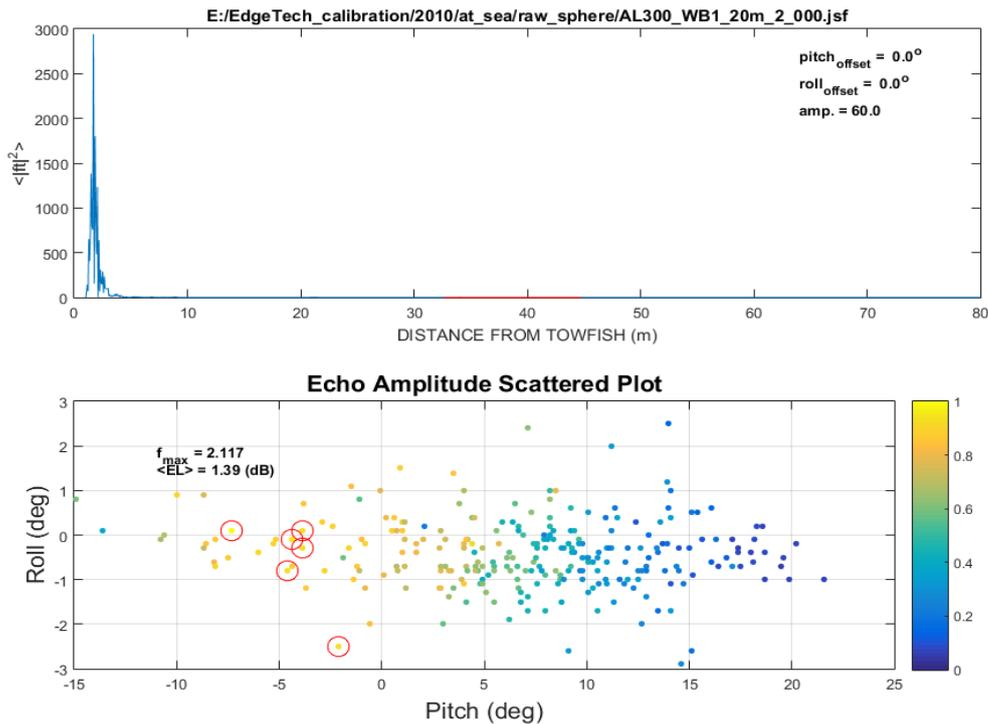
Figure 12. Second output diagram of plot2d\_color script used during calibration. The top plot depicts an average ping, with the red marking signifying the data being analysed. The bottom plot show the individual pings plotted according to the pitch and roll of the system, with the colour signifying intensity of the signal. Pings selected for further processing are circled in red.
