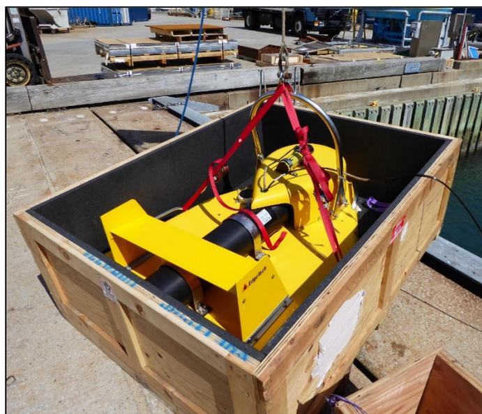
Figure 3. Marlab EdgeTech 3200 being hoisted from its storage box during a test calibration procedure.
