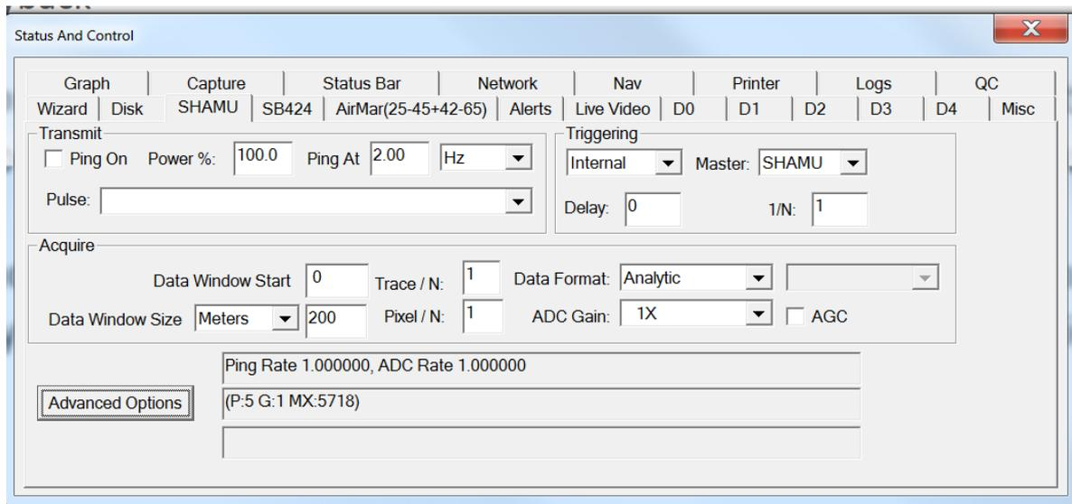
Figure 10. Control panel of JSTAR used to control the for one of the transducers (in this case SHAMU). This is where the pulse is selected, and the ping timings are set. Controls for activating the pinging are also present. Each of the transducers has its own separate set of controls.
