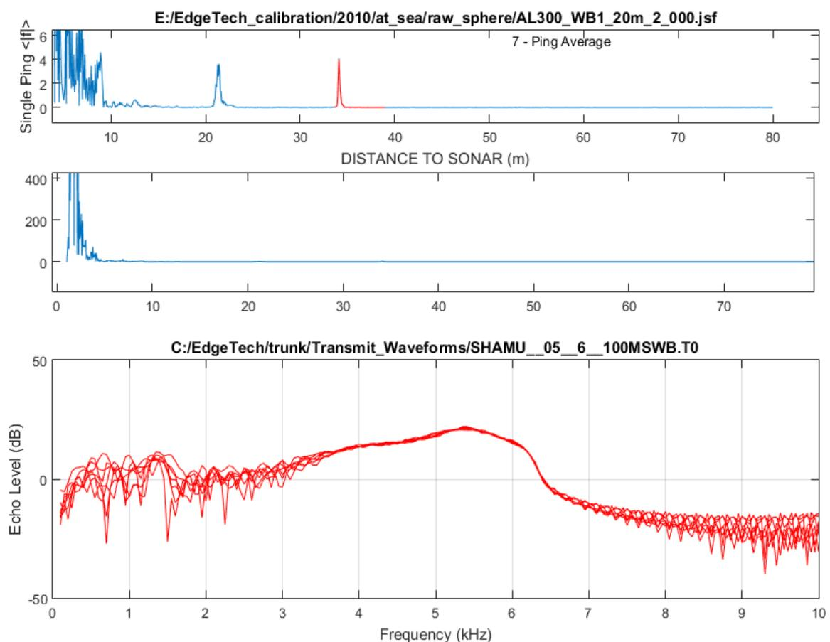
Figure 13. Output of `get_system_response`, final stage of calibration. The top plots show a single and averaged pings respectively (from the ones chosen by `plot2d_color`), with the first one being magnified. The bottom show a frequency-domain plot of the selected pings. Of primary interest is the tight grouping of pings between 3.5 kHz and 6.5 kHz – the aim of the final selection is to get this as smooth as possible.
