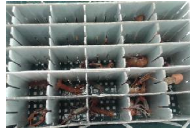
Figure 9-1: Tube-set boxes with different sizes of internal compartments used in the preliminary survival trial. Left panel: small (3x3 cm); central panel: medium (10x3 cm) and right panel: large (10x6.5 cm).
