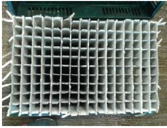
Figure 9-1: Tube-set boxes with different sizes of internal compartments used in the preliminary survival trial. Left panel: small (3x3 cm); central panel: medium (10x3 cm) and right panel: large (10x6.5 cm).
