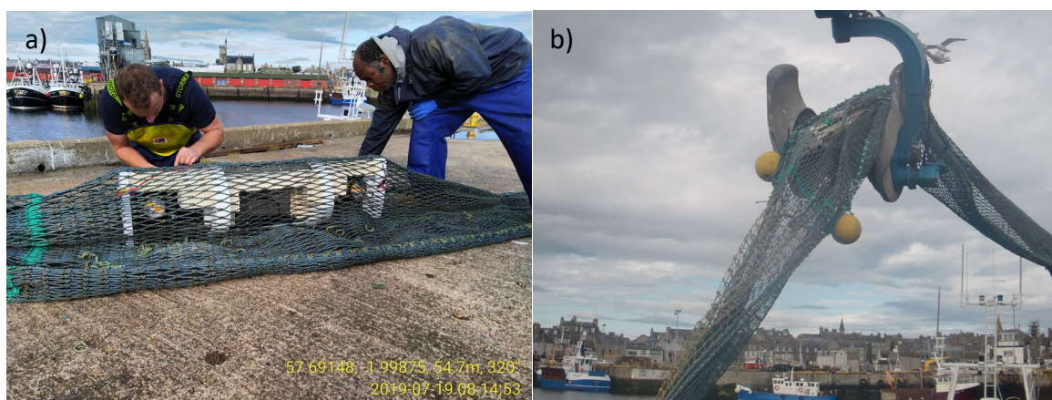
Figure 3. a) Inserting the camera frame into the trawl extension. b) the net with the frame being lifted by the vessel's power block
