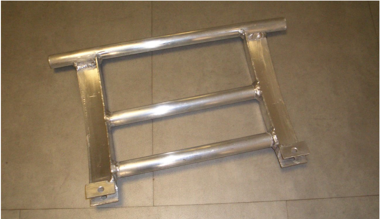
Figure 11 Frame for the modem transmitter fabricated using aluminium alloy
