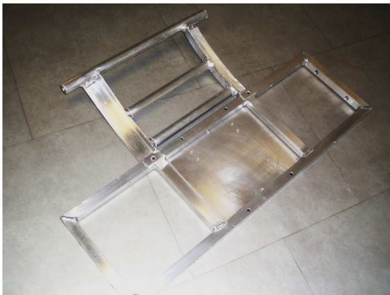
Figure 13 Assembled frame of the modified stereo camera frame and modem transmitter
