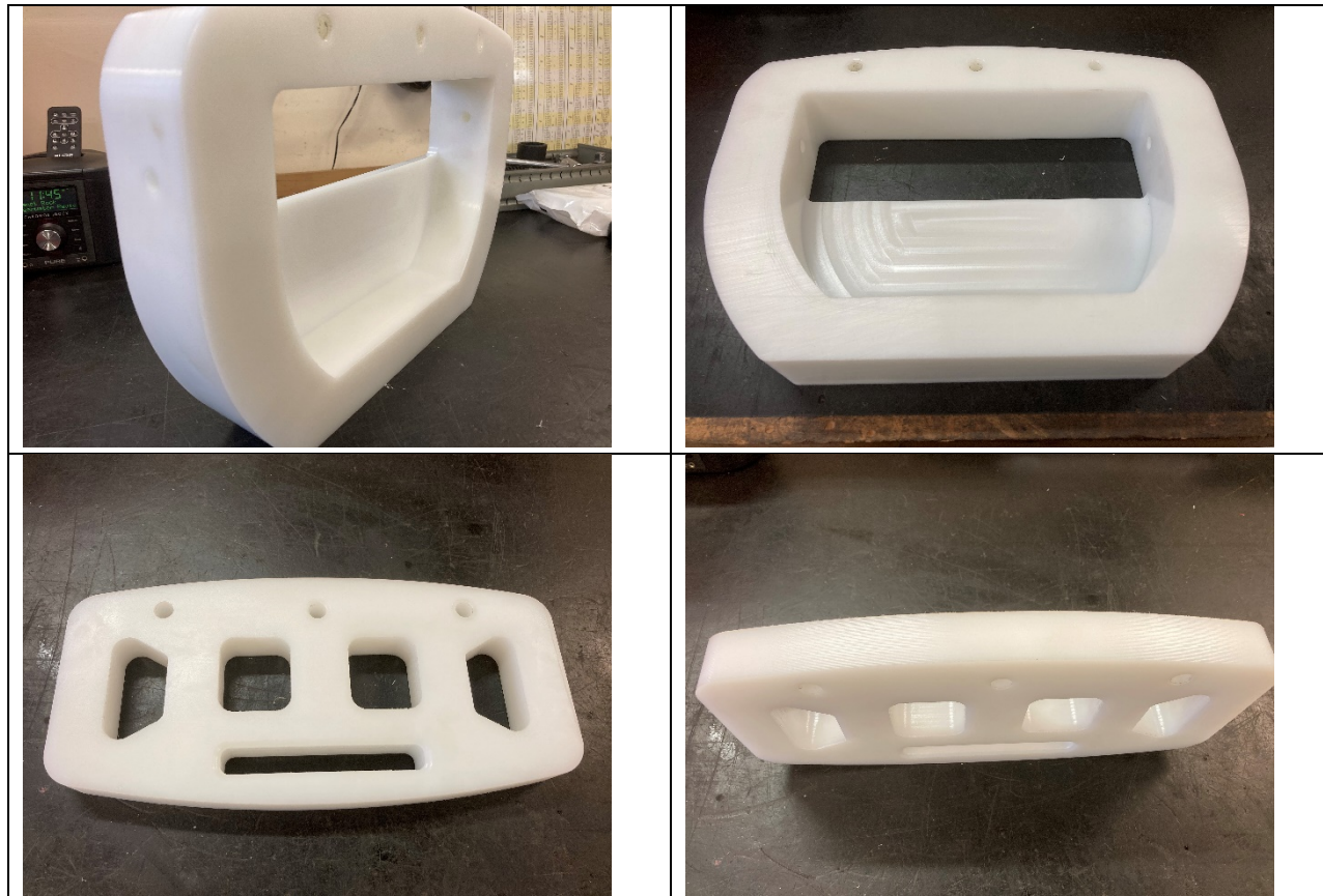
Figure 14 HDPE parts of the stereo camera frame fabricated using CNC machining
