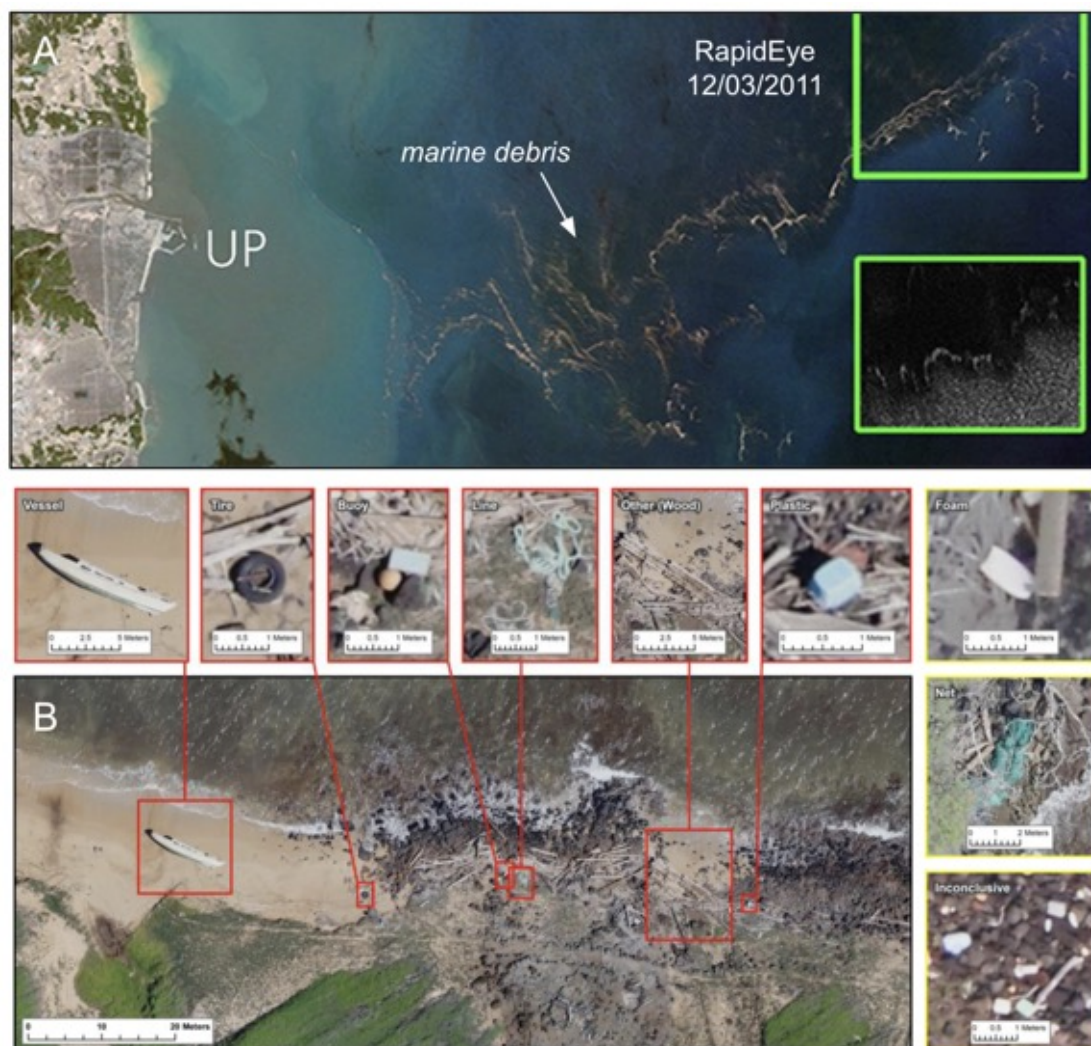
Figure 14. High resolution imagery of marine debris from (a) RapidEye (modified from Ref 30 ) and (b) aerial surveys using a Cessna 206 plane (Ref 32 )
