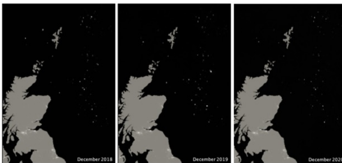
Figure 21. Nighttime monthly composites east of Scotland from VIIRS, showing bright lights from cities, on land, and in the sea from vessels (including shipping) and oil/gas infrastructure.
