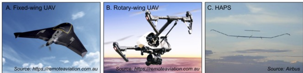
Figure 3. Example (a) fixed and (b) rotary-wing UAVs; (c) high altitude pseudo satellite (HAPS)
