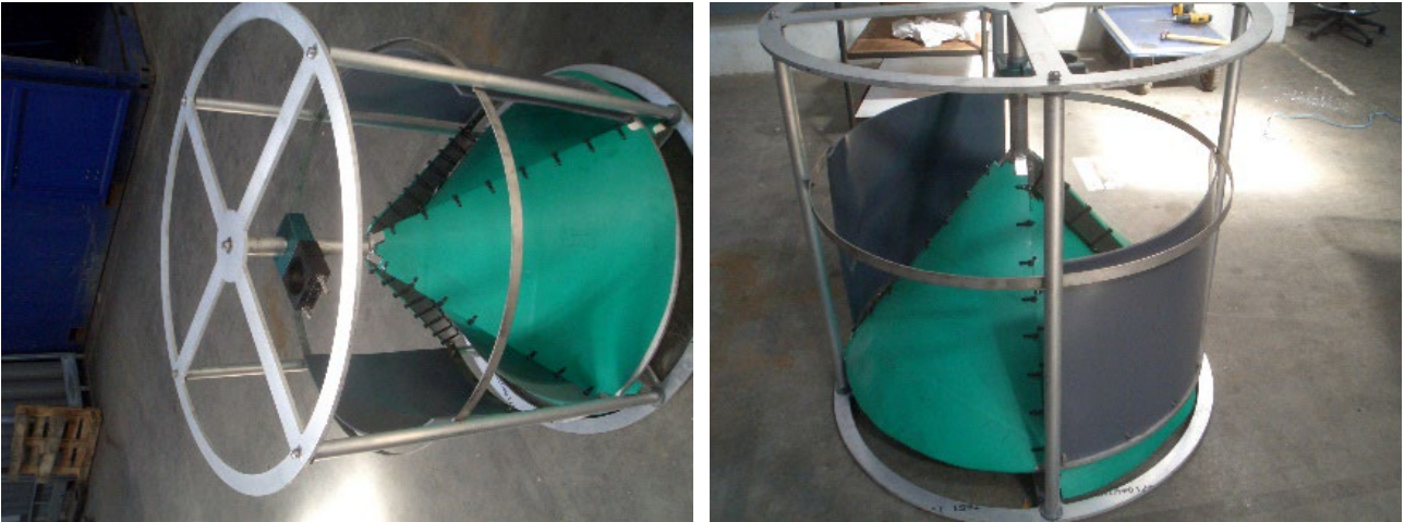
Figure 9 Version 3 of the prototype in release position (cones closing off the cod end which would be to the right-hand side of the left image and beneath the lower part of the right image). The conical sections (in green) and doors (in grey) were made from high density plastic.
