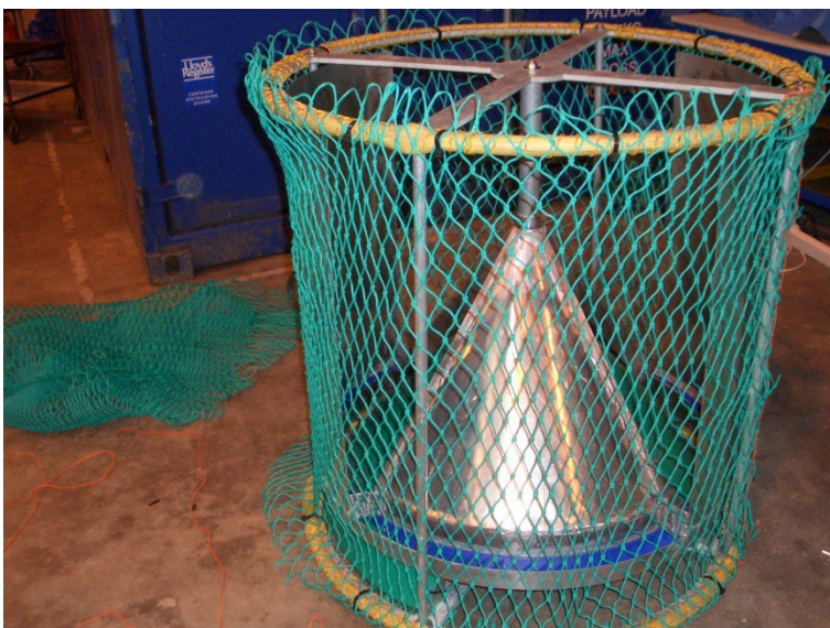
Figure 12 Version 4 of the prototype with new aluminium cone sections and hydrodynamically operated blades (in blue).
