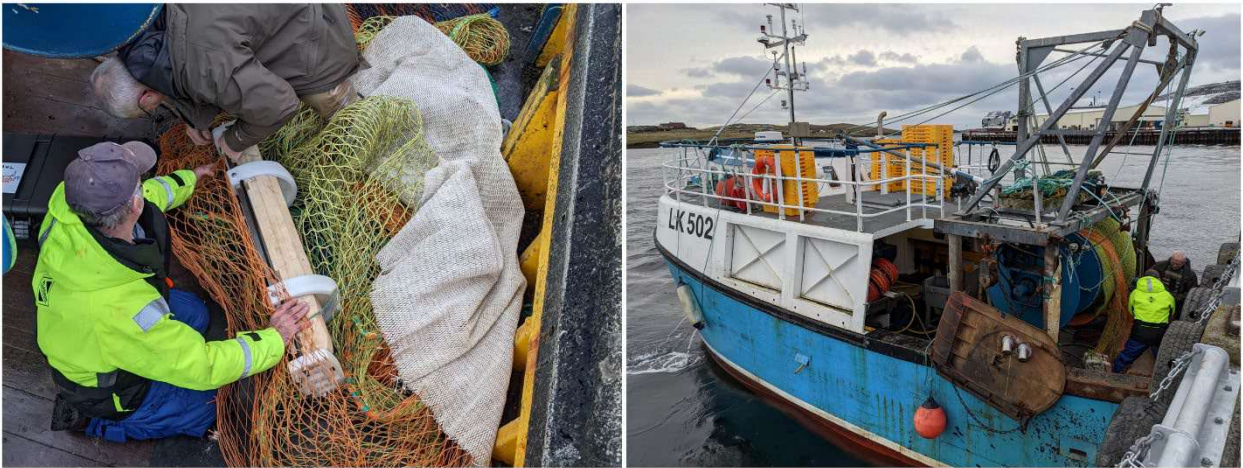
Figure 50. Rigging white netting into net extension aboard Atlantia II .
