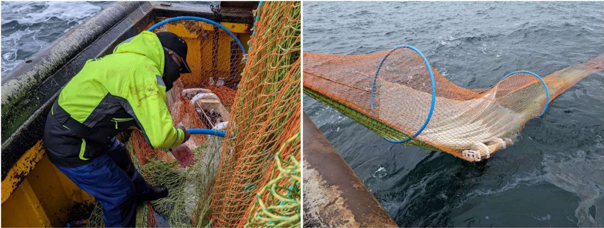
Figure 52. Attaching and deploying MDPE piping in the net extension.
