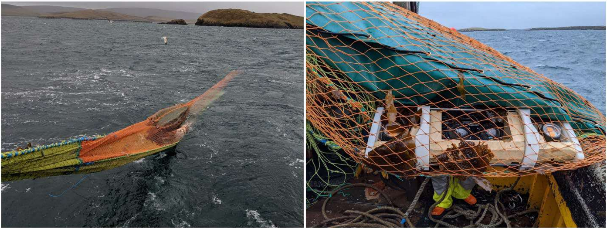
Figure 56. Deploying and recovering the stereo camera with pipes removed during D6.
