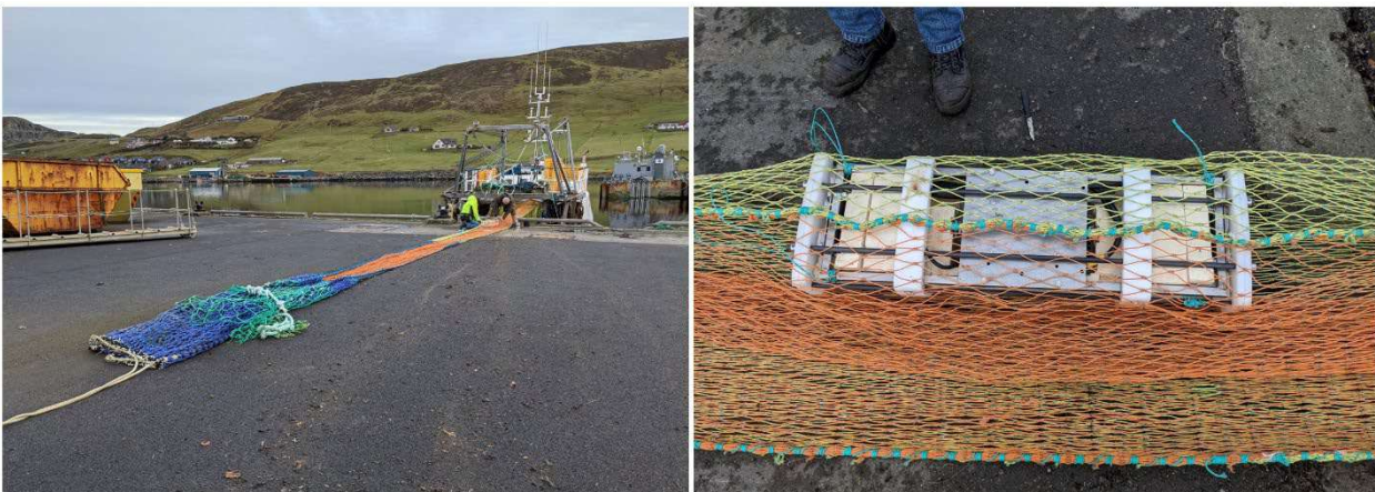
Figure 48. Attaching stereo camera system to the rock hopper net aboard Atlantia II .
