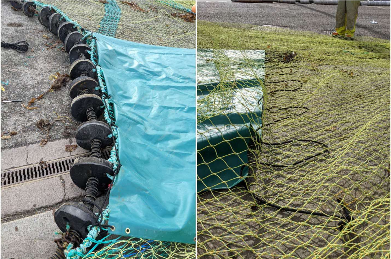
Figure 81. Detail of SSS rigging to footrope (left) and at trailing edge (right) following further alterations prior to D22.
