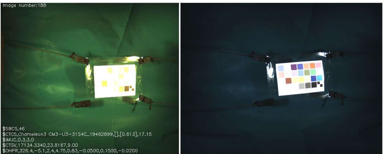
Figure 62. Colour card images during tank tests with default settings (left) compared to initial adjusted settings (right).
