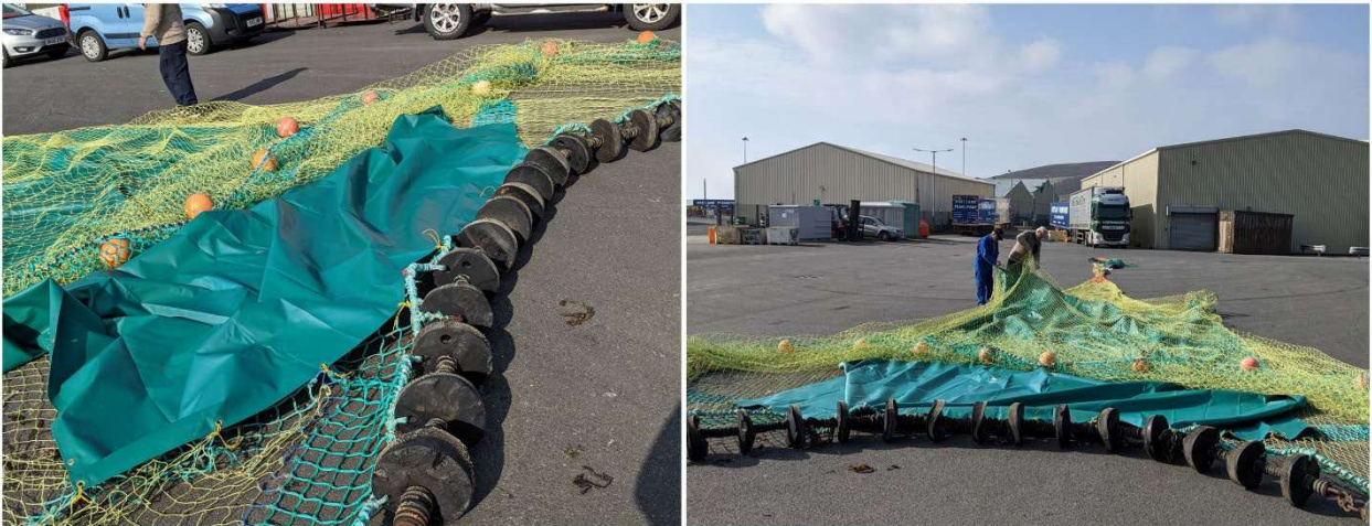
Figure 73. Initial fitting of the SSS to the gear.
