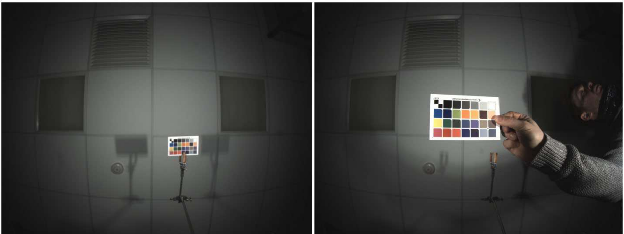
Figure 63. Example stereo camera images from subsequent bench tests using lower exposure settings.
