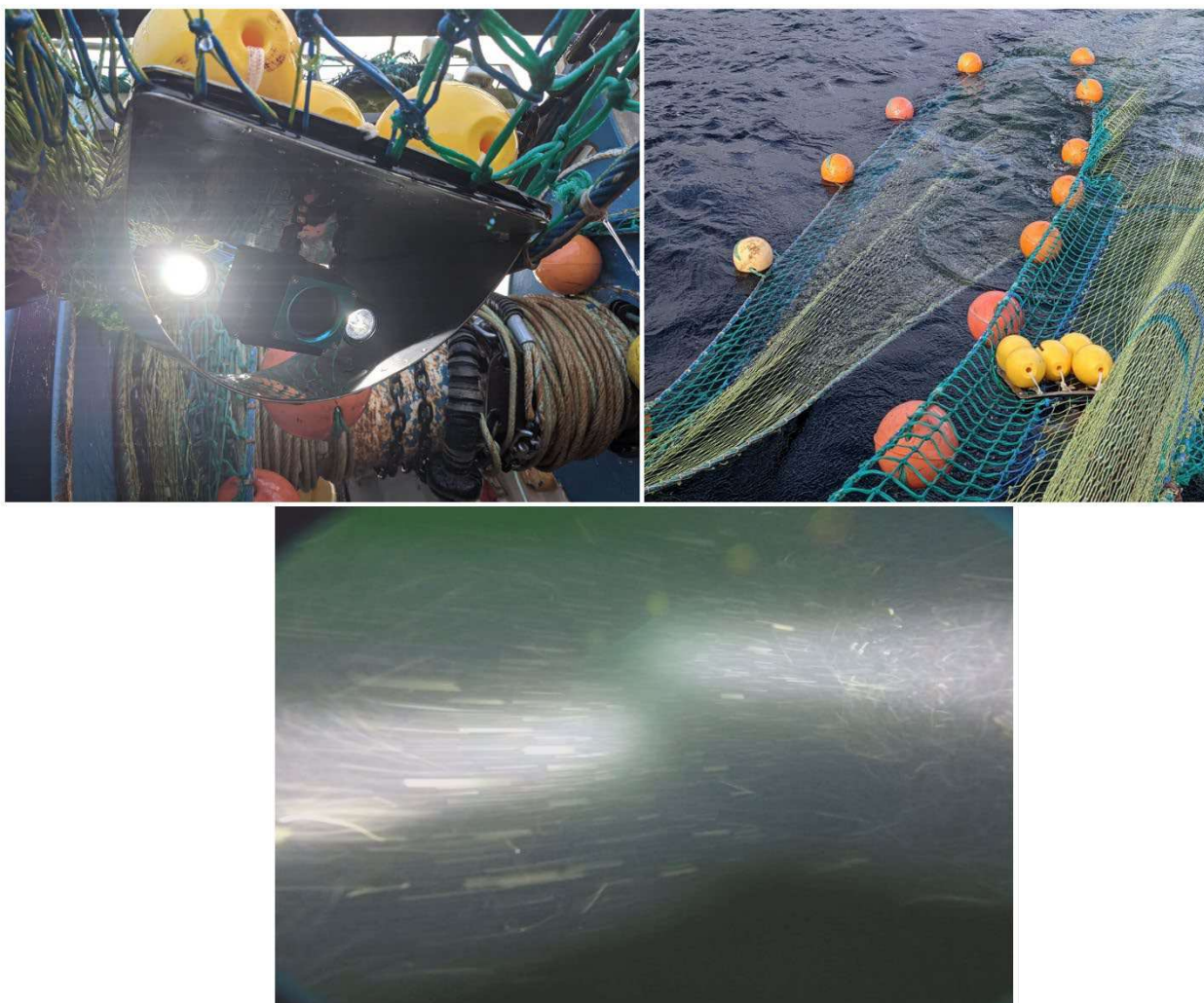
Figure 75. Rigging of GoPro camera housing during D19 to inspect mouth of net (top figures) and example screenshot from resulting video (bottom figure) showing poor visibility and high levels of backscatter with headline and ground gear faintly visible.
