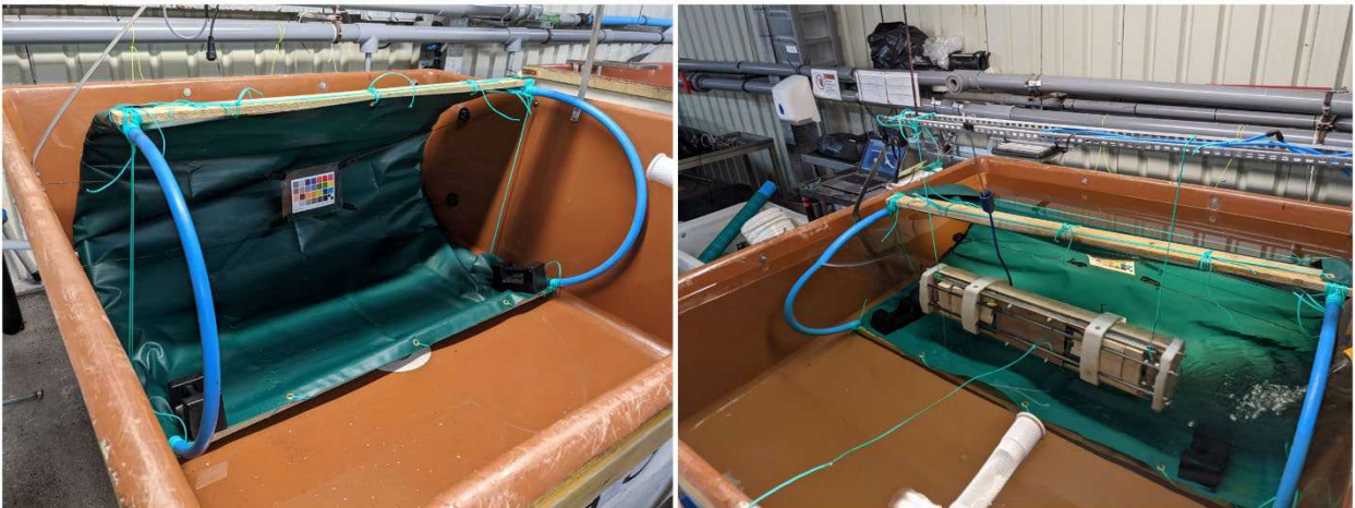
Figure 61. The tank and test rig used for underwater adjustments prior to being filled with water (left) and later during adjustments (right).
