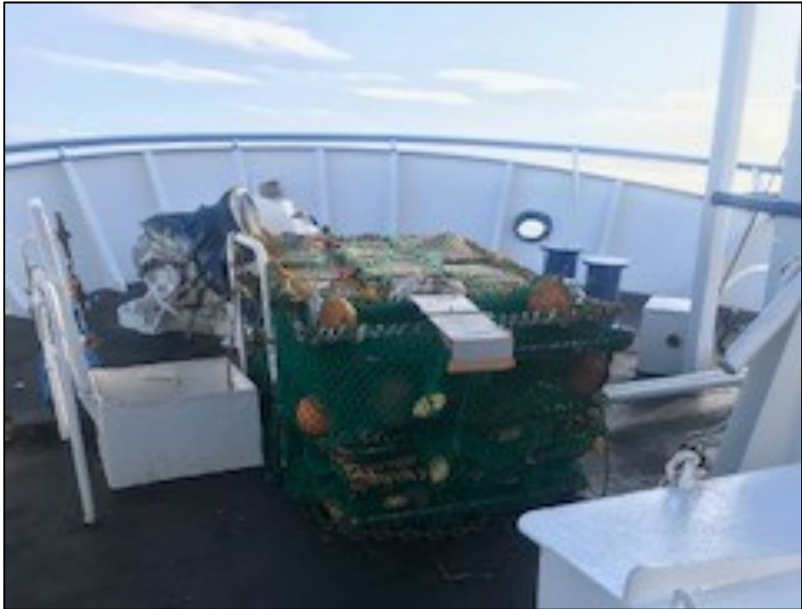
Figure 4: Fleet of eight traps compact and stowed on deck of the Carina .
