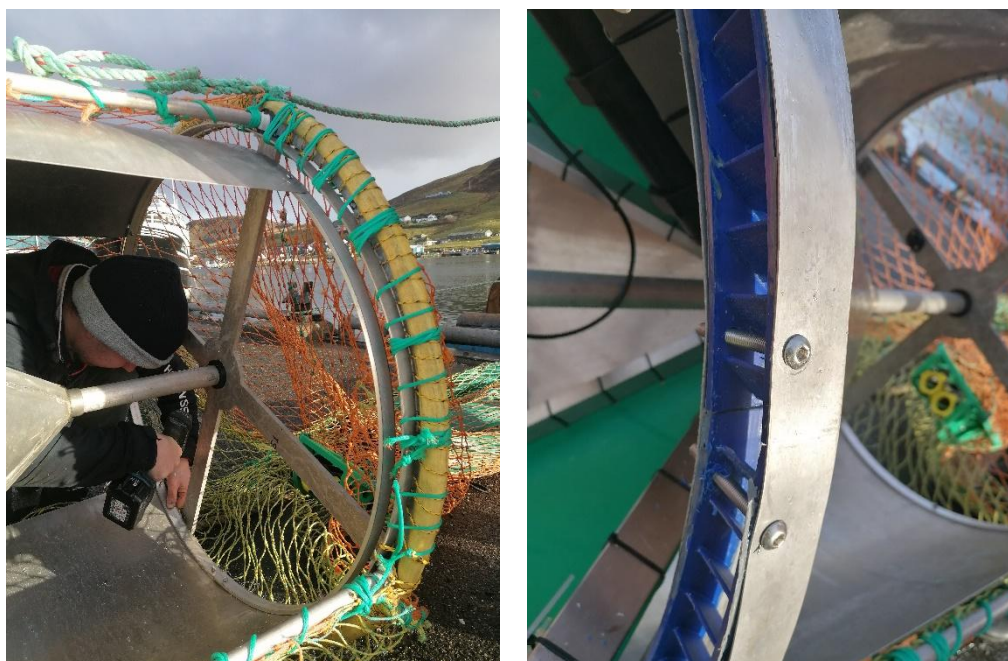
Figure 8 – Gate repairs. Left – addition of metal internal ring to strengthen doors with three bolts secured per door. Right – Long bolts placed through metal bordering and radial fins along the whole circumference of the cone.
