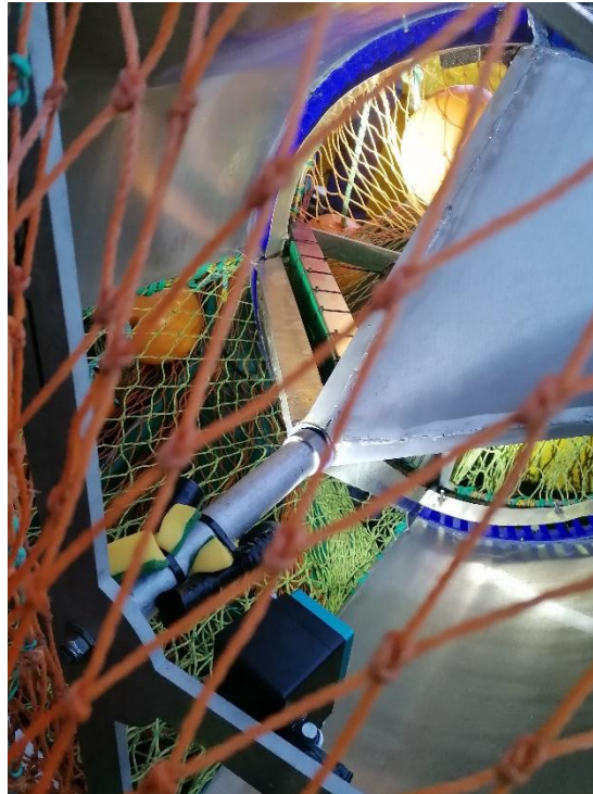
Figure 9 – Two torches and a GoPro were set up at the base of the gate. Torches cable tied to shafts with sponges to angle torches.
