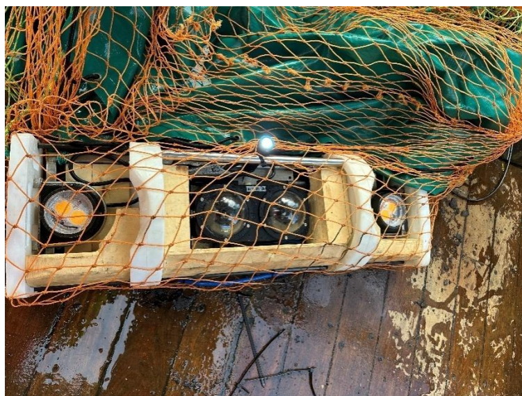
Figure 41 – Dive torch rigged to stereo camera frame to ensure illumination in case strobes were not flashing.
