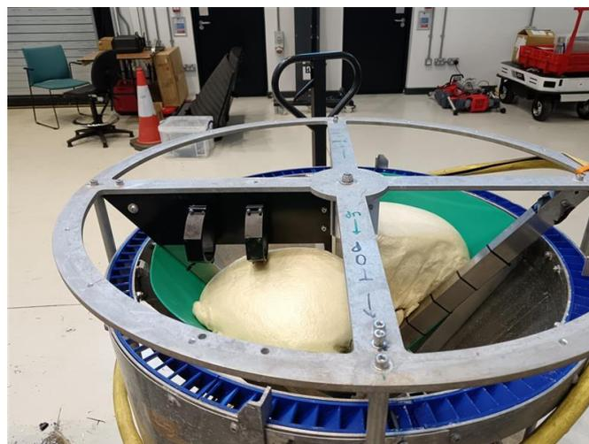
Figure 17: (Gate V2) latch bottle relocation & buoyancy foam
